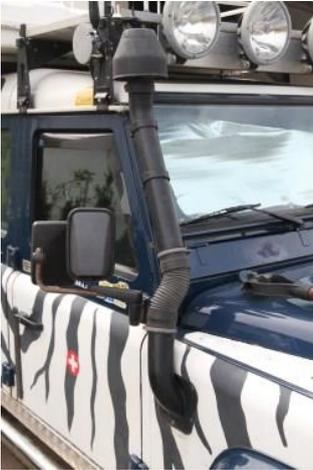
In Offroading, snorkels are used on the one hand to raise the air intake for the engine so that deeper wading is possible. On the other hand, they are also used to filter out dust particles to keep them away from the air filter (i.e. desert sand).
