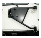
My Zebra is robustly built and can withstand alsmost all adversenesses. But the spare wheel at the rear door? Mounted on 3 mm steel sheet? And that with underdesigned hinge-joints? In rough environment?
