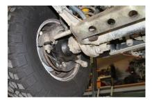
As a broken or deformed steering link by stones, rocks or simply muddy terrain can be quite dangerous, a respective protection should be simply standard for Offroaders in my opinion. En route, it is almost impossible to fix a steering link. This is the reason why some people always carry a spare steering link with them. However, I do not, as this adds again weight to my already overloaded Zebra.
