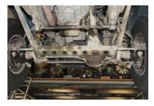
being damaged is accordingly high. However, a decision has to be made between steering link protection and antiroll bar (stabilizer) as mounting both can lead to interference with the axle articulation (to be checked out).
