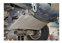
An underride protection at the front of the car is indispensable and belongs to the standard equipment of an Off-Roader. And I do not mean these ornamental protection plates that look very shiny but are of no use. An underride protection must be built as solid as a rock so that it can withstand the massive impact-energy when necessary.
