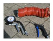
I have two sets of tubes with me. One fort he quick and dirty case and one spiral coiled tube with manometer for exact inflation. Further, I always carry with me a blow-out gun. It can be very helpful in cleaning the air filter on long and dusty tours. The pressure in the spiral coiled tube is enough to provide short air blasts. Apart from saving costs and space for a spare filter, it is also light weighted.
